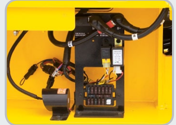
A concentrated Fuse Box for Easy Inspection
