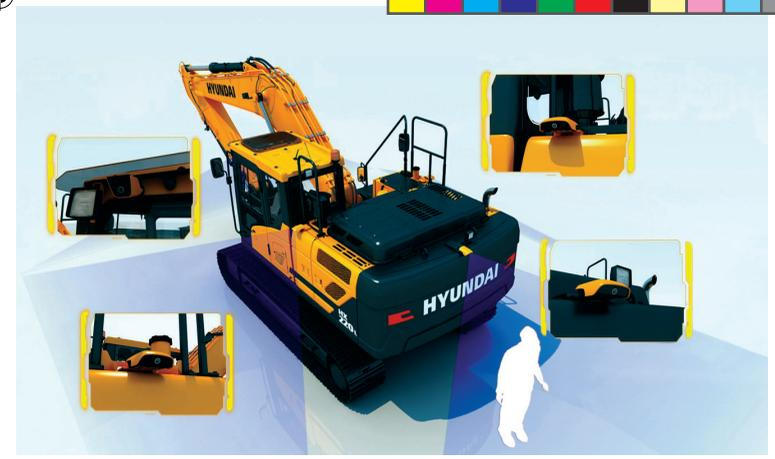
The AAVM option combines images from four external cameras to provide 360° virtual operating view.
