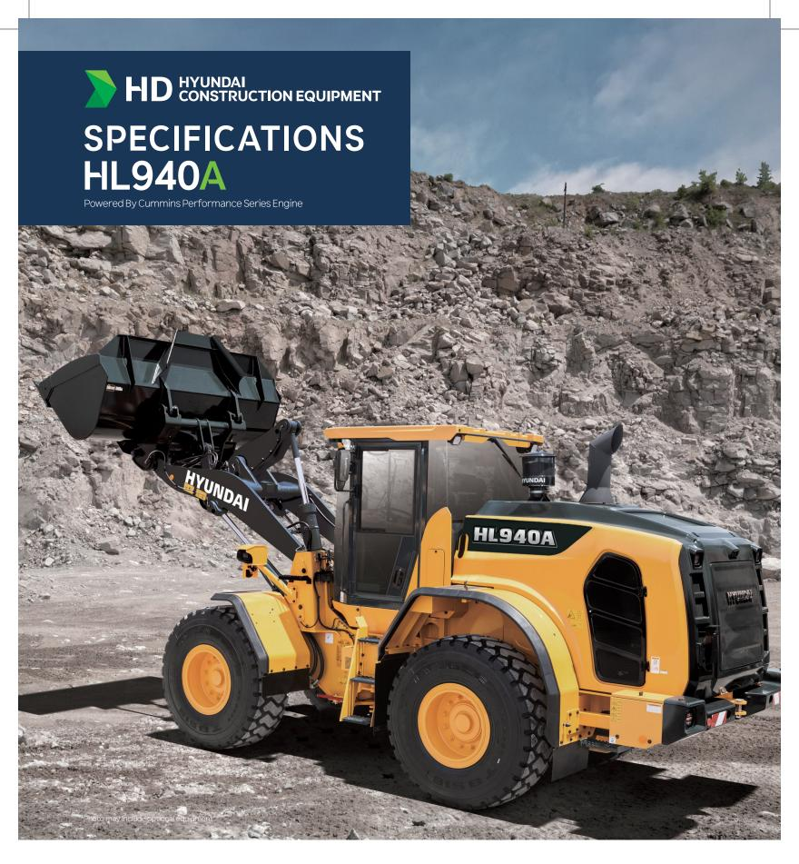
**Net Power** 154 hp (115 kW) at 2,200 rpm Operating Weight 29,985 lb (13,601 kg) -30,560 lb (13,862 kg) Standard Bucket 3.0 yd³ (2.3 m³)
