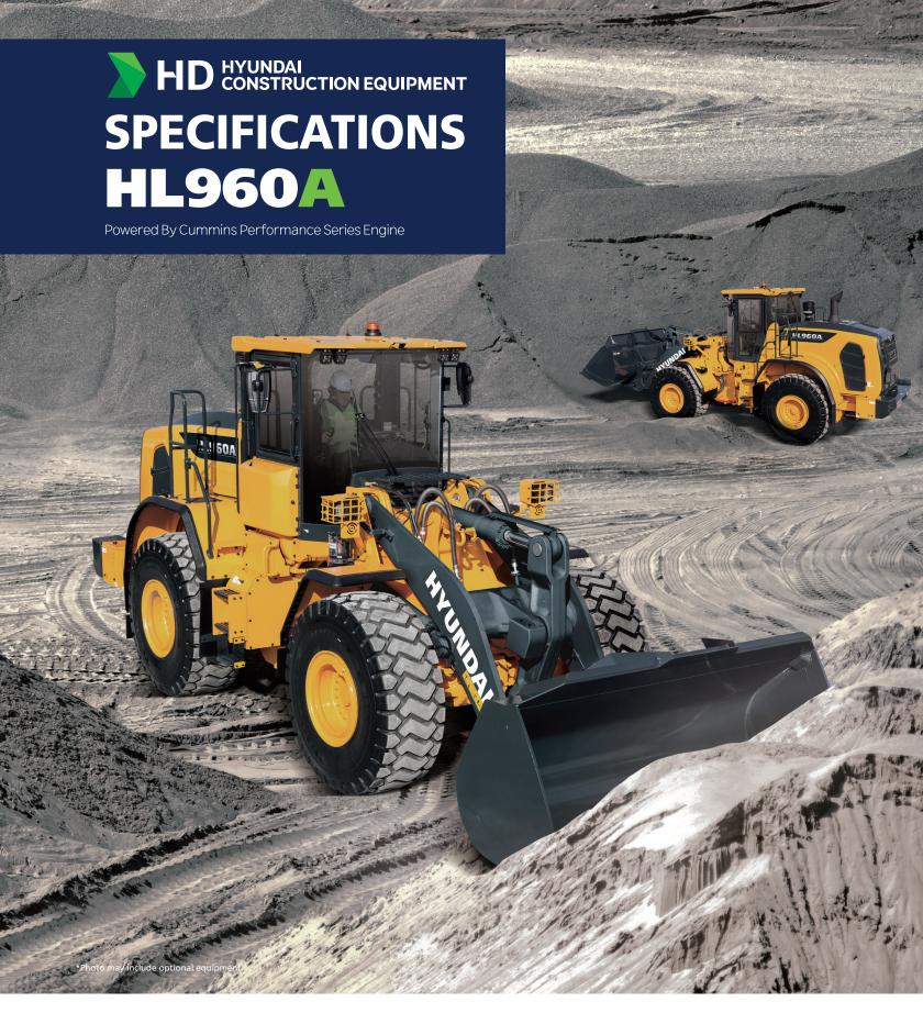
**Net Power** 222 HP (166 kW) at 2,200 rpm Operating Weight 19,831 kg (43,720 lb) -20,031 kg (44,160 lb) Bucket Capacity 3.3 m<sup>3</sup> (4.3 yd<sup>3</sup>)
