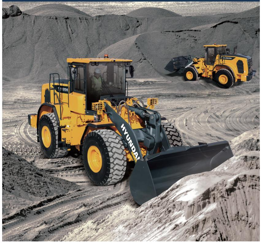
**Net Power** 222 hp (166 kW) at 2,200 rpm **Operating Weight** 42,880 lb (19,450 kg) – 44,710 lb (20,280 kg) Bucket Capacity 4.32 yd<sup>3</sup> (3.3 m<sup>3</sup>)
