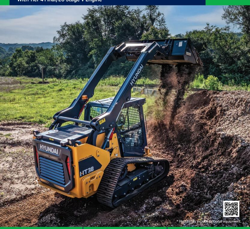
Engine Gross Power 115.3 HP (86 kW) / 2,400 rpm Rated operating capacity (35% of tipping load) 3,806 lb (1,727 kg) Operating Weight 12,785 lb (5,799 kg)
