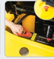
Battery Disconnect Lever / Switch
