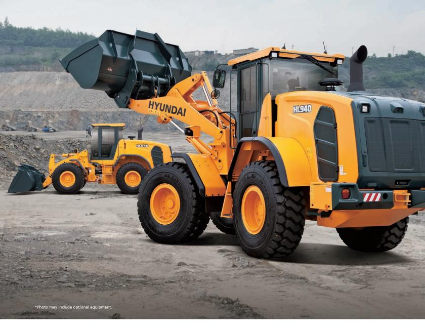
**Net Power** 156 HP (116 kW) / 2,100 rpm **Operating Weight** 13,300 kg (29,321 lb) **Standard Bucket** 2.3 m<sup>3</sup>/ 3.0 yd<sup>3</sup>
