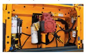
To achieve optimum precision, Hyundai redesigned the hydraulic system to provide the operator with super fine touch and improved controllability. Improved pump flow control reduces flow when controls are not being used to minimize fuel consumption.
