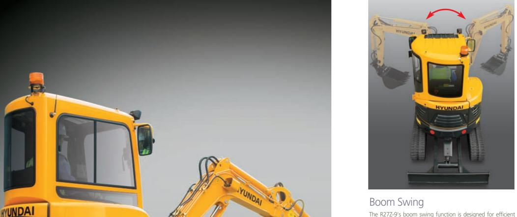
The R27Z-9's boom swing function is designed for efficient work in congested residential and urban areas. The boom can be offset left or right within an operating range.
