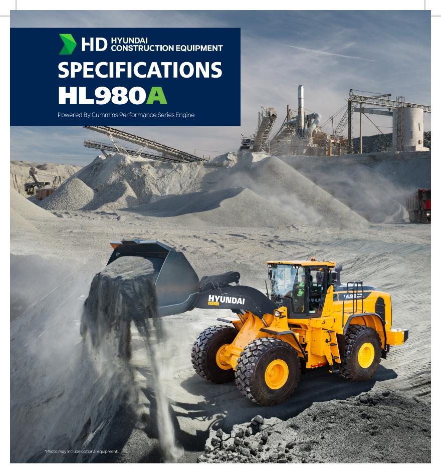
**Net Power** 351 HP (262kW) 2,000 rpm Operating Weight 31,352 kg (69,120 lb) -31,502 kg (69,450 lb) Bucket Capacity 5.6 m<sup>3</sup> (7.3 yd<sup>3</sup>)
