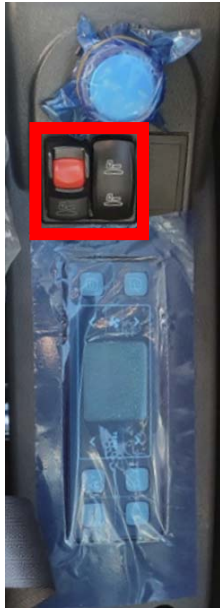
Elevating cab switch
