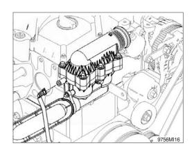
② Install the cap. Operate the engine until it reaches a temperature 80°C (176°F), and check for coolant leaks.
