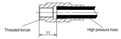
③ Assembly the ferrule insert with the threaded ferrule and the high pressur hose : Grease or oil on thread of the ferrule and the conical end of the ferrule insert good and screw the ferrule insert in the assembled ferrule.
