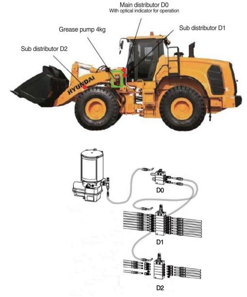
\* Refer to the CENTRAL GREASE LUB SYSTEM of parts manual for detail.
