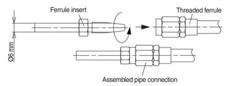
\* The dimensions of the hoses are able to differ in a slight range. If the diameter are smaller as standard, the ferrule can be push on the hose without power and without rotary motion. Remedy:
