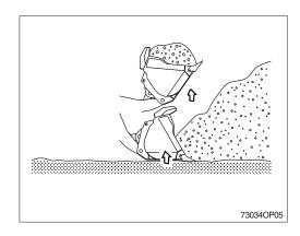
When it is difficult to dig into the soil, move the bucket control lever forward and backward to move the bucket teeth up and down.
