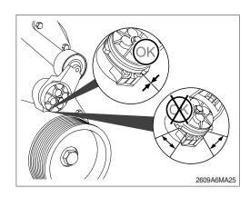
(4) Check the location of the drive belt on the belt tensioner pulley. The belt should be centered on, or close to the middle of, the pulley. Misaligned belts, either too far forward or backward, can cause belt wear, belt roll-offs, or increase uneven tensioner bushing wear.
