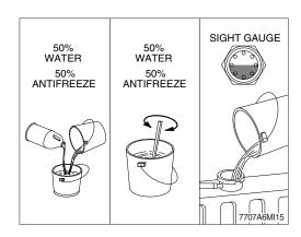
\* The system must be filled properly to prevent air locks. During filling, air must be vented from the engine coolant passages.
