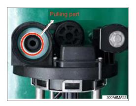
(4) Replace the filter and fit with a new filter.
