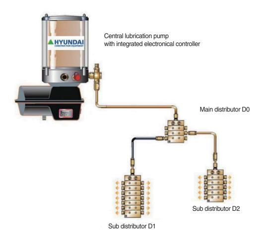
The progressive system supplies the lubrication points in a fixed order.
