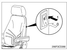
① The seat heater can be turned on/off by pressing the switch.
