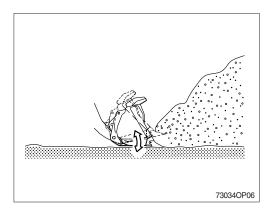
If the machine operates with its front tires lifted, its driving force will deteriorate and excessive force will be applied to the rear tires. Avoid operating in that posture.
