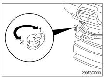
① The absorber setting of the seat can be varied to suit the on and off-road working conditions.
