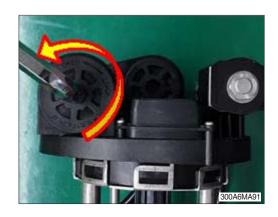
(3) Pull out the filter by using a long nose pliers.
