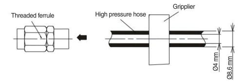
② Stick on the high pressure hose with a gripplier and grease or oil the end of this very good. The threaded ferrule turn on the hose left-turning up to the dimension in the sketch (11 mm).
