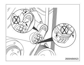
(2) With the belt installed, verify that neither tensioner arm stop is in contact with the spring case stop.
