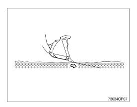
② Advance the machine and lift the bucket using the bucket control lever to dig out the soil.
