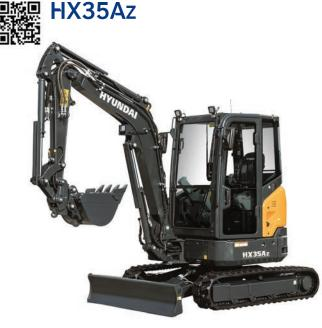
Net power Kubota D1703 24.2 hp (17.8 kW) @ 2,200 rpm
