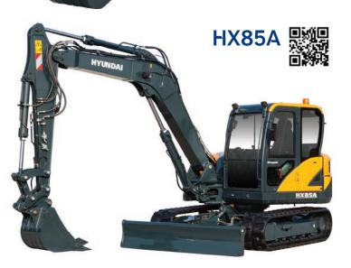
**Net power** Yanmar 4TNV98C-PHYB 65.1 hp (48.5 kW) at 2,400 rpm
